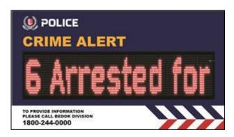
The LED Crime Alert Singage aims to raise crime awareness and deter would-be criminals from committing shop theft. The signage can easily be setup and is able to display eyecatching text in various languages. The text can also be changed instantly through a secured Wi-Fi connection.
