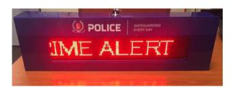
The Electronic Message Board (EMB) is portable and lightweight and can be setup easily at the lift lobby. The EMB can be programmed up to eight messages in various languages.
