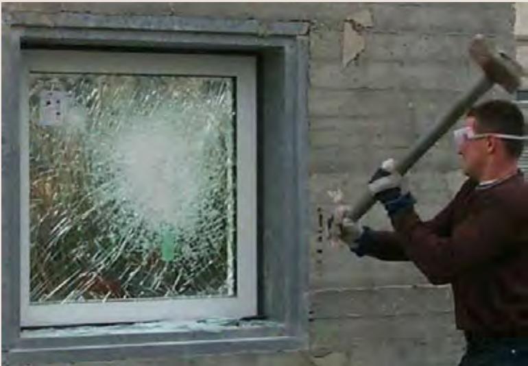
Figure 37: Testing of 15 minutes forced entry resistant window
