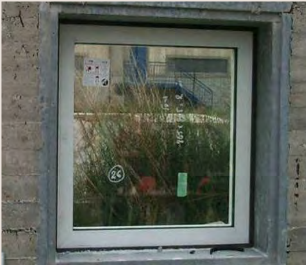
Figure 36: Window before forced entry testing
