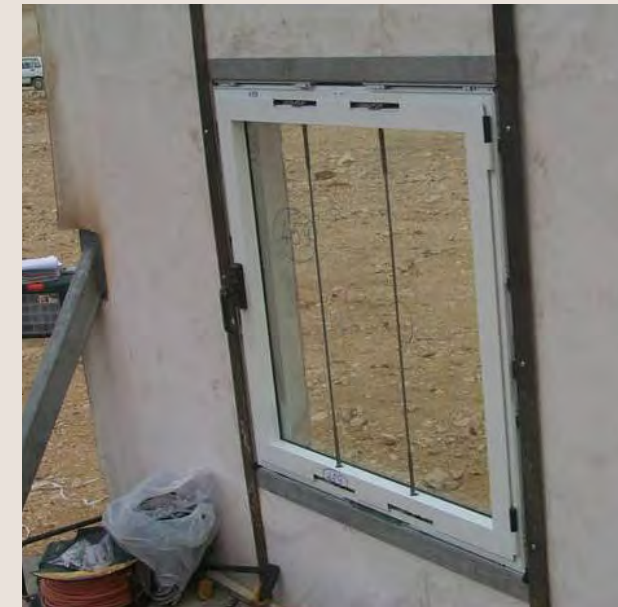
Figure 28: Cable protected window for low blast levels (before explosion)
