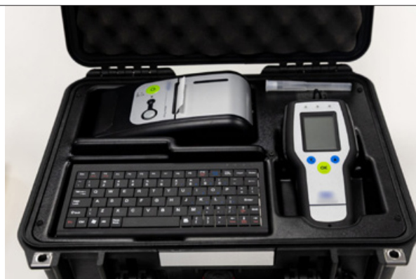
The HBEA (trial model shown) is a portable device that instantly records and prints out a motorist's breath alcohol concentration.
