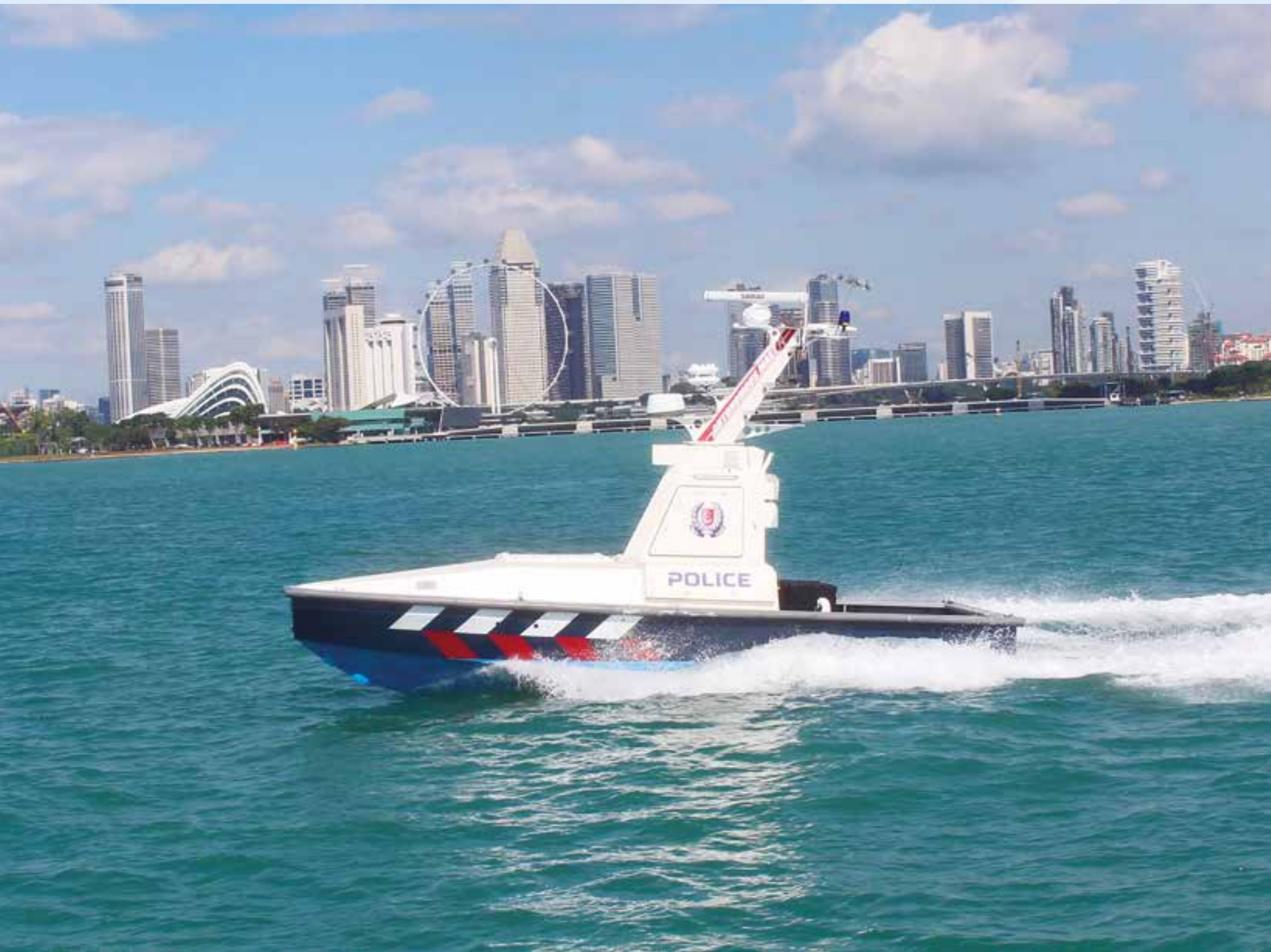
The Unmanned Surface Vessel can patrol Singapore waters autonomously over a set route, and can help project police presence and detect any intrusions.
