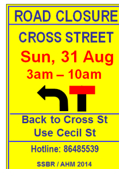
Figure 4 Example of lane closure sign
