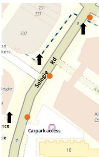
Figure 10 Another example of lighting placement along lane closure
