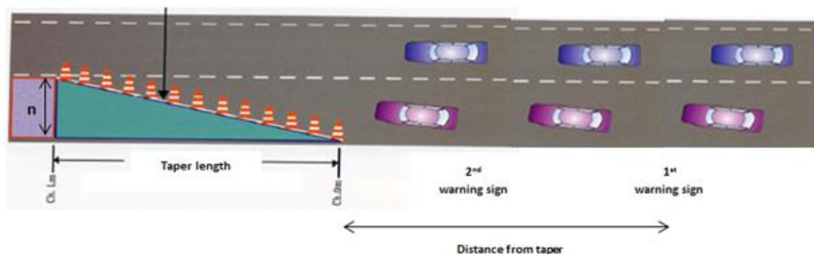
Figure 2 Taper length and sign distance (illustration)
